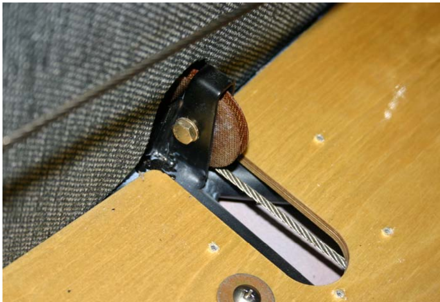
FIGURE 2 – Cover Removed-Inspection of Pulley Diameter
