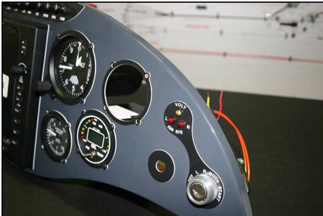
FIGURE 5 - New Amber LED Light Installed
