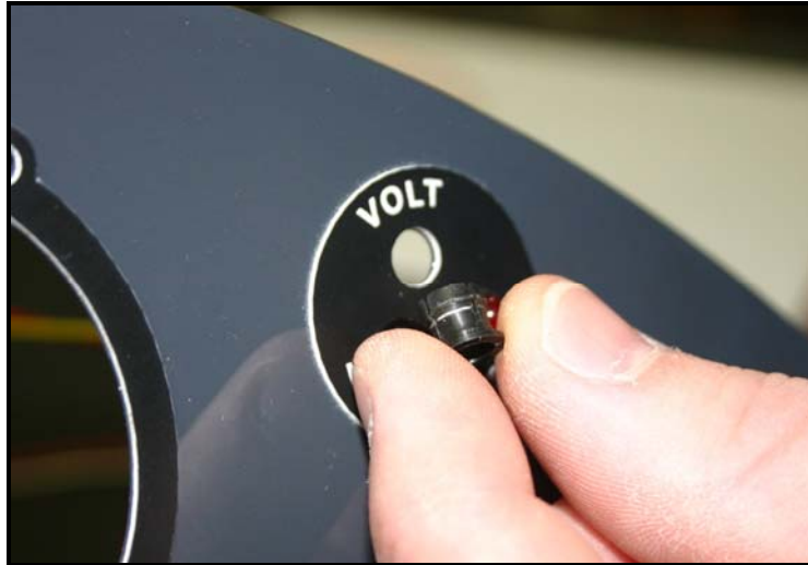
FIGURE 2 - Inner Ring Installation
