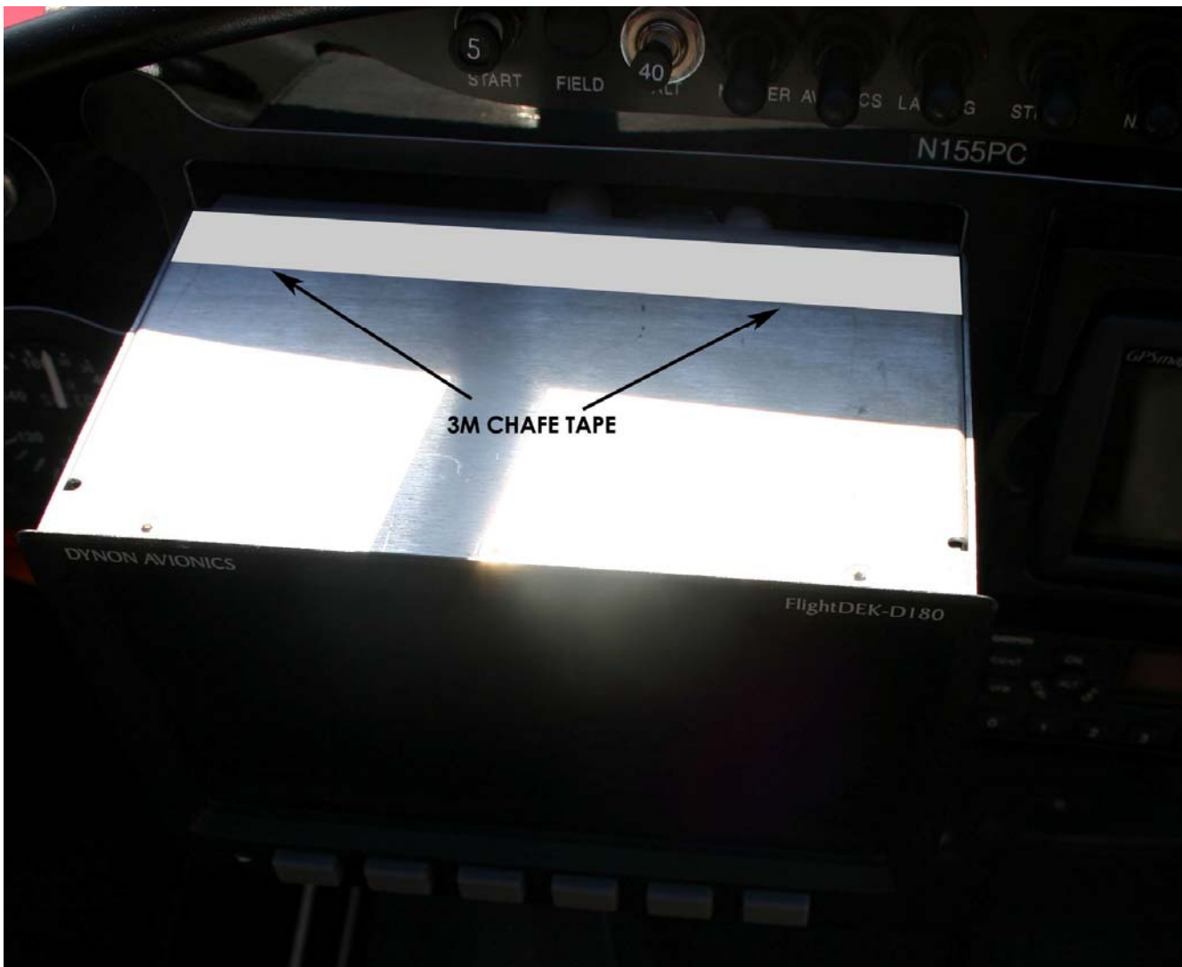
Figure 3 - Upper part of Dynon with chafe tape installed
