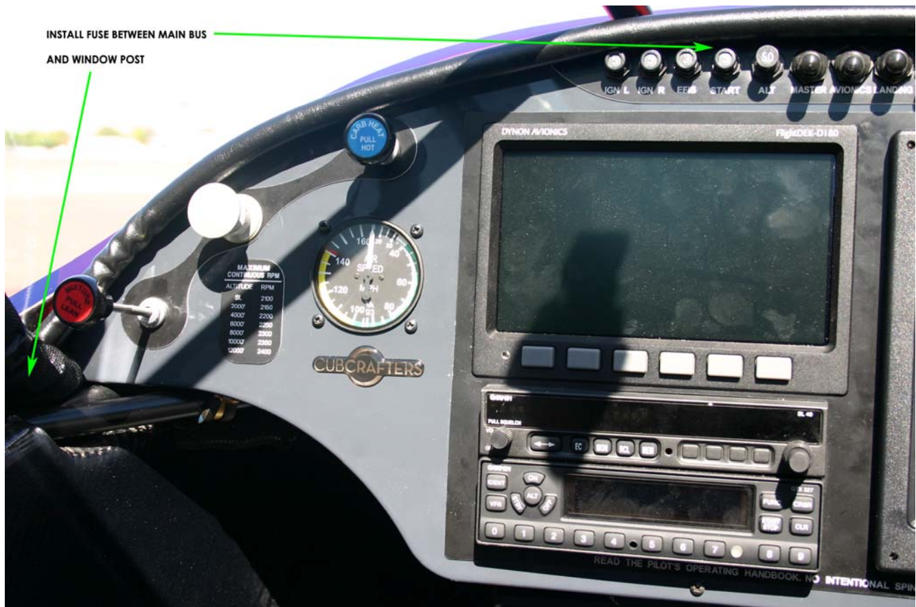
Figure 7 - Location of fuse holder and fuse
