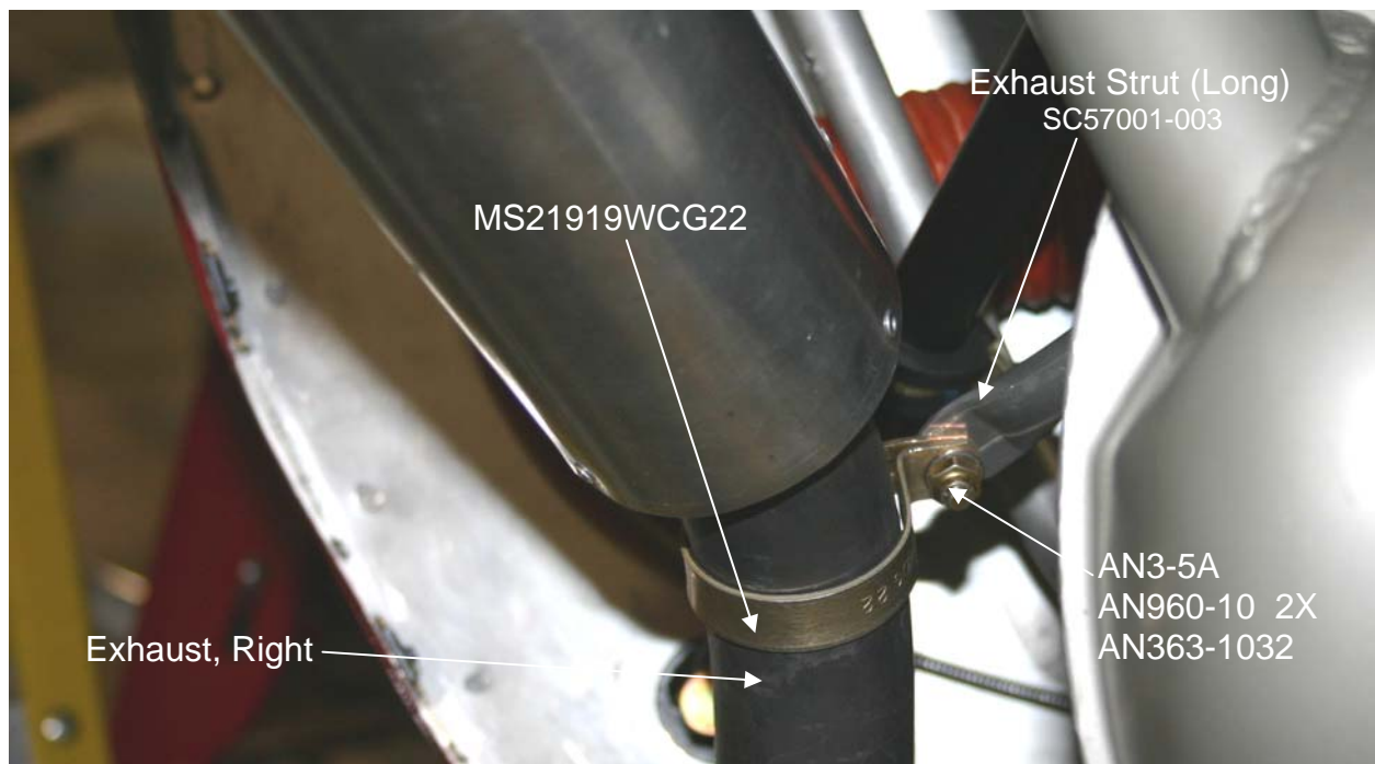
Figure 3 – Right Exhaust Strut Attachment to Oil Pan
