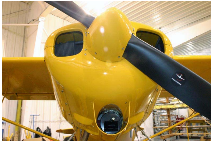
Figure 1 View looking at airbox with filter removed
